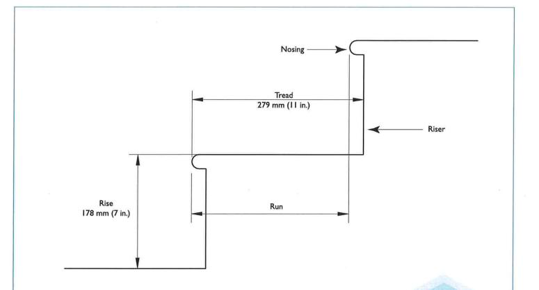
Figure 1: Suggested Dimensions for the Elements of a Step
