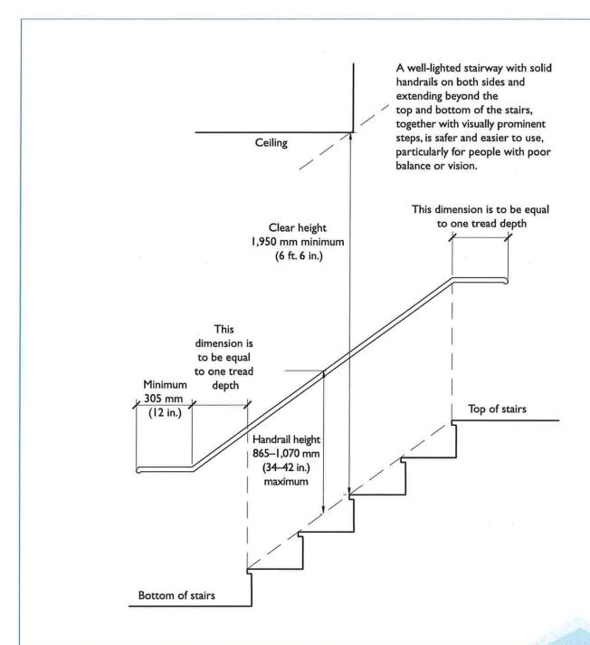
Figure 2: Suggested Dimensions for the Elements of a Stairway
